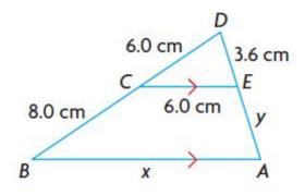
A new bridge is going to be built across a river, but the width of the river cannot be measured directly. Surveyors set up posts at points A, B, C, D, and E. Then they took measurements relative to the posts.
