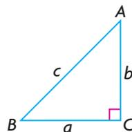
In any right triangle, there are three primary trigonometric ratios that associate the measure of an angle with the ratio of two sides. For example, for  $\angle ABC$ , in Figure 1,
