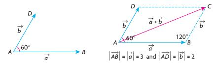
To calculate the value of  $|\vec{a} + \vec{b}|$ , draw the diagonal of the related parallelogram. From the diagram,  $\overrightarrow{AB} + \overrightarrow{BC} = \vec{a} + \vec{b} = \overrightarrow{AC}$ . Note that the angle between  $\overrightarrow{AB}$  and  $\overrightarrow{BC}$  is 120°, the supplement of 60°.
