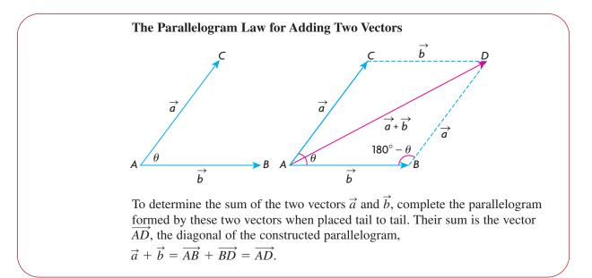
Consider the triangle formed by vectors  $\vec{a}$ ,  $\vec{b}$  and  $\vec{a} + \vec{b}$ . It is important to note that  $|\vec{a} + \vec{b}| \le |\vec{a}| + |\vec{b}|$ . This means that the magnitude of the sum  $\vec{a} + \vec{b}$  is less than or equal to the combined magnitudes of  $\vec{a}$  and  $\vec{b}$ . The magnitude of  $\vec{a} + \vec{b}$  is equal to the sum of the magnitudes of  $\vec{a}$  and  $\vec{b}$  only when these three vectors lie in the same direction.
