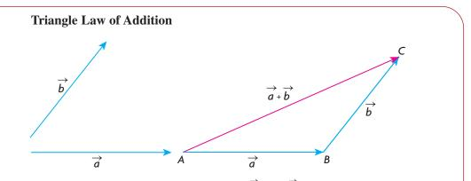
In the diagram, the sum of the vectors  $\vec{a}$  and  $\vec{b}$ ,  $\vec{a} + \vec{b}$ , is found by translating the tail of vector  $\vec{b}$  to the head of vector  $\vec{a}$ . This could also have been done by translating  $\vec{a}$  so that its tail was at the head of  $\vec{b}$ . In either case, the sum of the vectors  $\vec{a}$  and  $\vec{b}$  is  $\vec{AC}$ .
