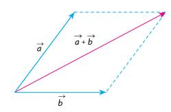
• The sum of the vectors  $\vec{a}$  and  $\vec{b}$  is also found by translating the tail of vector  $\vec{b}$  to the head of vector  $\vec{a}$ . The resultant is the vector from the tail of  $\vec{a}$  to the head of  $\vec{b}$ .
