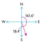
Other ways of stating this would be  $E71.6^{\circ}S$  or a **bearing** of  $161.6^{\circ}$  (i.e.,  $161.6^{\circ}$  rotated clockwise from due North).
