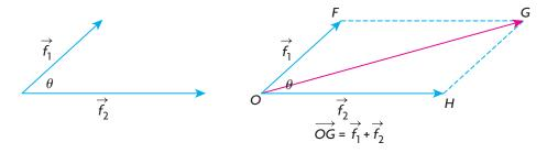
The length (or magnitude) of each vector representing a force is proportional to the actual force exerted. After the tugboats exert their forces, the ship will head in the direction of  $\overrightarrow{OG}$  with a force proportional to the length of  $\overrightarrow{OG}$ .
