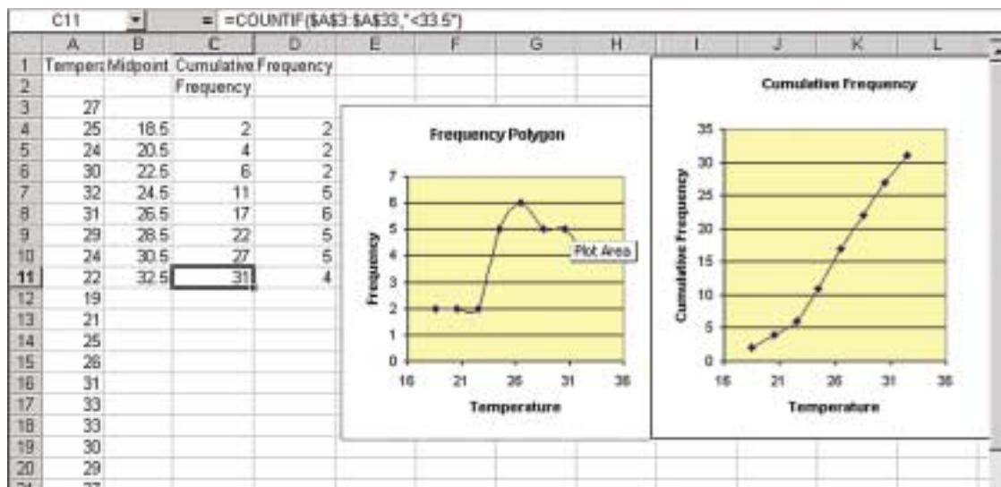
In Corel® Quattro® Pro, you can also use the Histogram tool in the Tools/Numeric Tools/Analysis menu to automatically tally the frequencies and cumulative frequencies.
