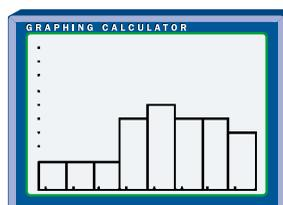
You can now use the **TRACE instruction** and the arrow keys to determine the tally for each of the intervals. Enter the midpoints of the intervals into L2 and the tallies into L3. Turn off Plot1 and set up Plot2 as an  $x$ - $y$  line plot of lists L2 and L3 to produce a frequency polygon.
