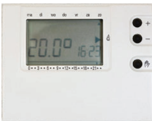
Figure 2 The sensor that measures the temperature in a digital thermostat is a thermistor. A thermistor is a resistor in which electrical resistance varies with changes in temperature.
